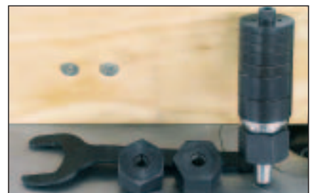
Machine spindle with holder for interchangeable spindles – 30 mm spindle and 8 and 12 mm standard collet holder
